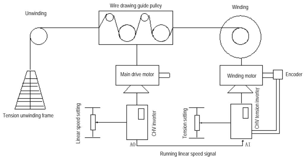
Schematic Diagram of CHV Winding Free of Tension Feedback
